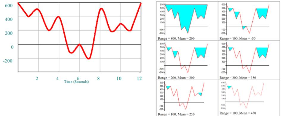
The stress range and its associated mean stress are determined from the load history shown in the graph. The load history is "filled with rain" in the graphed load history. After the stress range and mean have been determined, the "rain" is drained from the lowest point. The range and mean for each remaining portion of trapped "rain" is then determined. From the results, Miner's Rule can be applied, and the fatigue life calculated.
